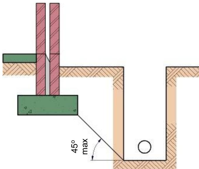
**Position of drainage trench near foundation**
